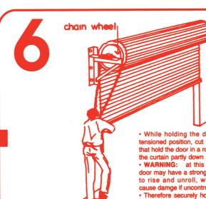
While holding the door in its tensioned position, cut the bands that hold the door in a roll and pull the curtain partly down as shown.
