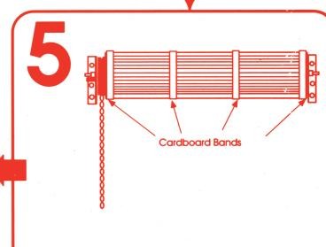
SPRING TENSIONING • Rotate the door one to two full turns in the direction of the arrow (shown in step 4)
